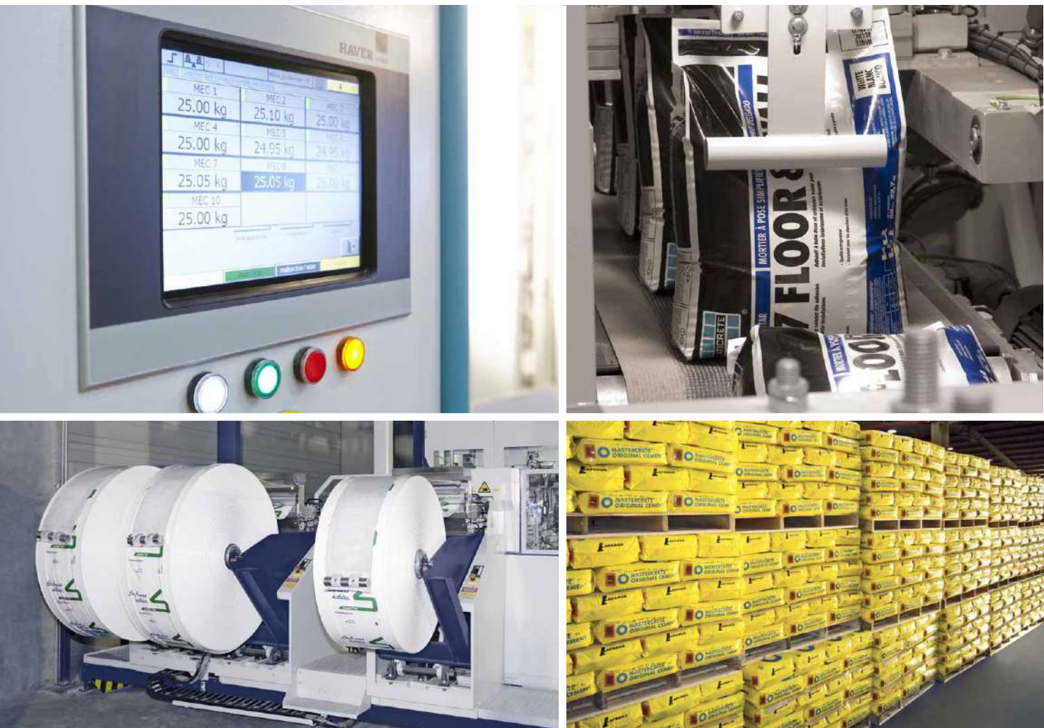
Weighing electronics MEC® with touch panel / Fully automatic Reel Changer Filled bag transport / Long shelf life – also outside
